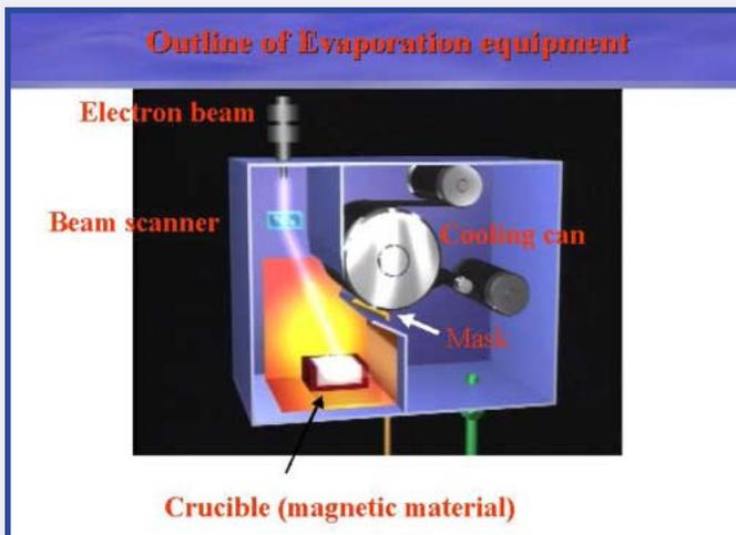
Sony introduced Metal Evaporated (ME) tape, the forerunner to AME tape, in 1989. It was first used in Sony Hi8 format video recording. Over the years, Sony has made improvements to the original ME tape that led to the introduction of the first-generation AME tapes in 1996 for data and video storage. A departure
